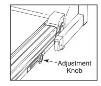
turn the knob clockwise. Note: The faster you run on the treadmill, or the more you weigh, the firmer the walking platform should be.
